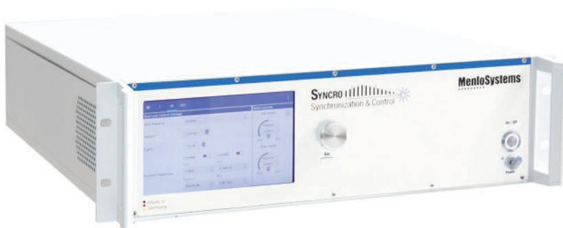
The RRE-SYNCRO features a dual channel PID controller, an integrated phase detector and integrated amplifier modules for the stabilization of the laser cavity, as well as integrated photo diode modules for laser repetition rate detection at fundamental and harmonic frequencies.
