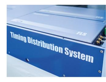
The main building blocks of the Timing Distribution System are an ultra low noise optical master oscillator that is synchronized to the master RF clock, a splitting and amplification unit to provide multiple optical signals to be distributed to the various clients, dispersion compensated fiber links, and detection and stabilization electronics to provide the error signals and the stabilization thereof.
