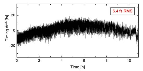
Out-of-loop long term timing drift between two stabilized fiber links:
