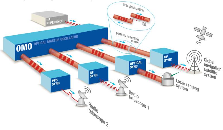
Scheme of a femtosecond synchronization system in operation at a geodetic observatory
