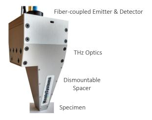
Menlo Systems provides a plug-in, compact terahertz reflection head with integrated optics for high-performance measurements with fixed working distance of 4" (~10 cm). The reflection head is suitable to all Menlo Systems terahertz timedomain spectrometers (THz-TDS) and contains 4 off-axis parabolic mirrors with focal lengths of 2" and 4", respectively.
