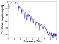
\*Typical terahertz reflective measurement using newest Menlo Systems' TeraSmart or TERA K15 showing timedomain signal and spectrum (50 ps scan window measured at 24 Hz).
