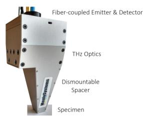
Menlo Systems provides a plug-in, compact terahertz reflection head with integrated optics for high-performance measurements with fixed working distance of 4" (~10 cm). The reflection head is suitable to all Menlo Systems terahertz timedomain spectrometers (THz-TDS) and contains 4 off-axis parabolic mirrors with focal lengths of 2" and 4", respectively.
