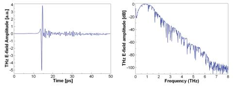
\*Typical terahertz reflective measurement using newest Menlo Systems' TeraSmart or TERA K15 showing timedomain signal and spectrum (50 ps scan window measured at 24 Hz).
