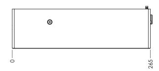
Technical drawing of the YLMO-930 laser head. The laser head comes equipped with detachable 25 mm posts and post clamps. Please contact us for more details and technical drawings of the control unit.
