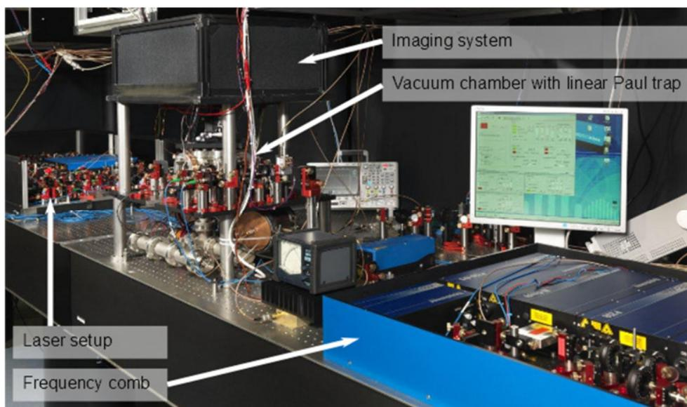
**Figure:** View of the experimental setup of the aluminum clock.
