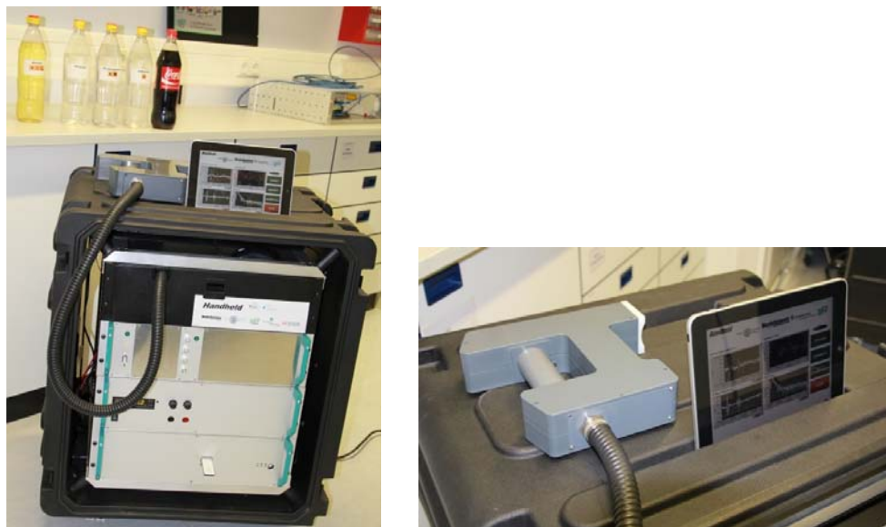
Figure 2: Handheld portable THz spectrometer for the detection of hazardous fluids (left picture) with measurement head (right picture)
