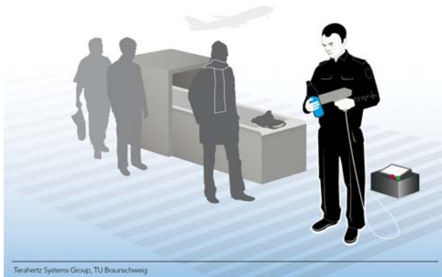
Figure 1: Handheld demonstrator of a THz detector for explosives identification
