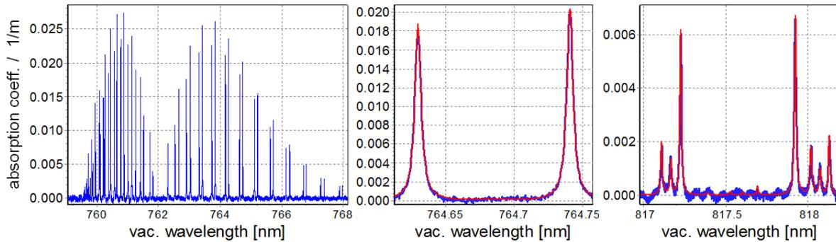
**Figure 4:** Example of an air absorption measurement for a 6.837 m interferometer arm displacement, the average result of 12 scans is shown. (a) Oxygen A-band at 762 nm. (b) Detail of the measured line profile (blue) compared with a model based on HITRAN data (red). (c) A few water vapor lines (78 % rel. humidity).
