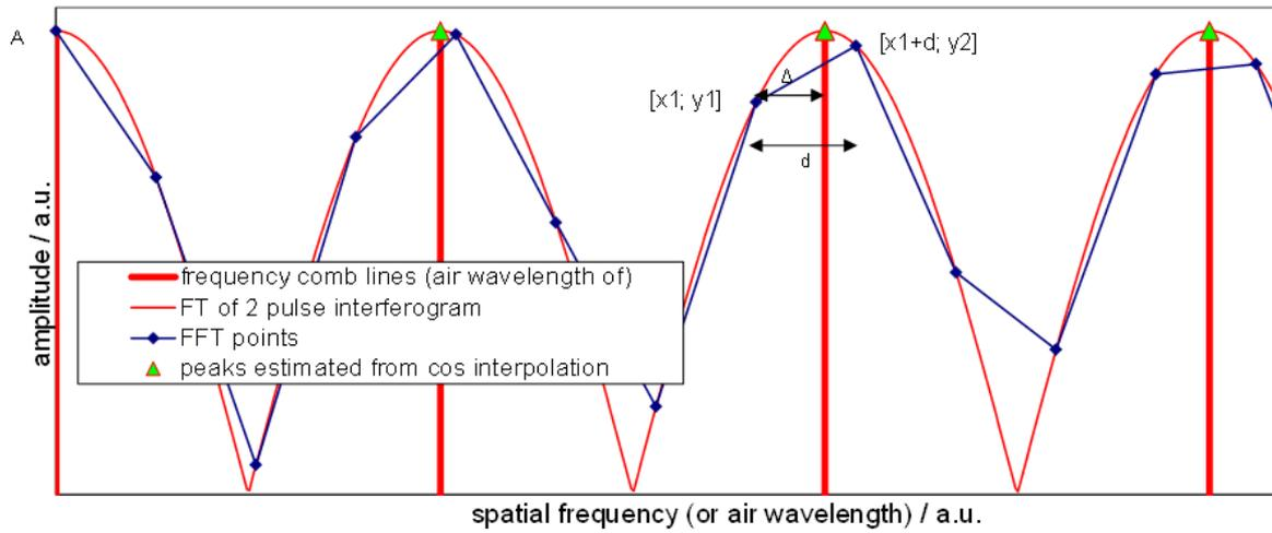
**Figure 1:** Illustration of amplitude and wavelength modelling of comb modes from FFT data calculated for an M=2 interferogram.
