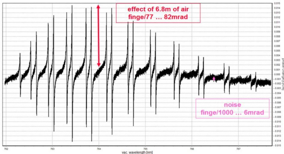
**Figure 7:** Change in spectral phase caused by 6.8 m displacement in air – average of 13 scans of O<sub>2</sub> at 765 nm.
