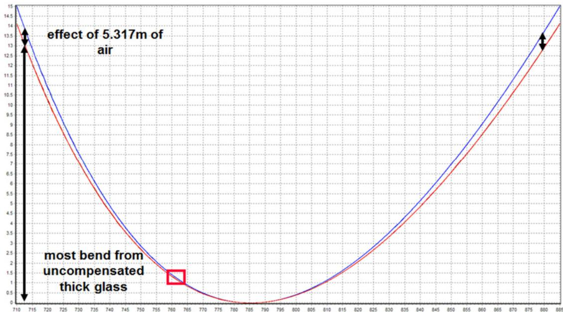
**Figure 6:** Spectral phase  $\sim$  second derivative of  $n(\lambda)$ : comparing spectral phase curves at the same stationary points of different pulses.
