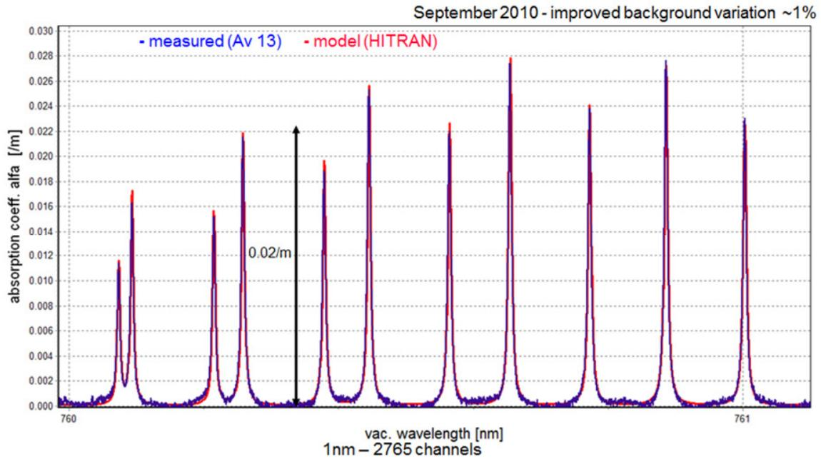
**Figure 5:** Detail of some O<sub>2</sub> lines from A-band at 762 nm, measured in 6.8 m of air.
