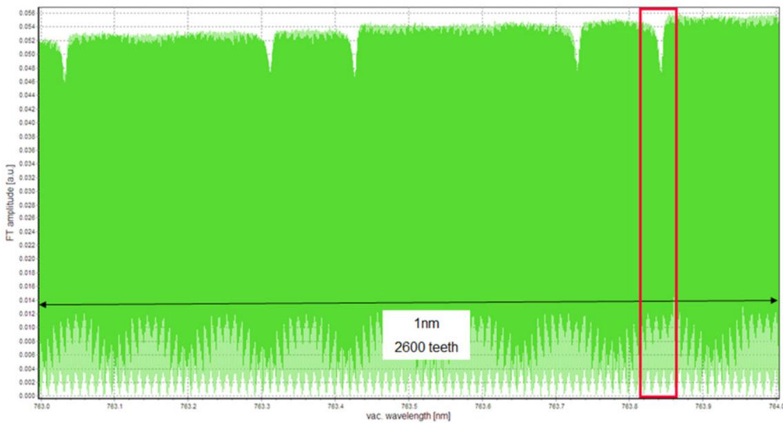
**Figure 2:** Raw FFT data: O<sub>2</sub> lines are visible
