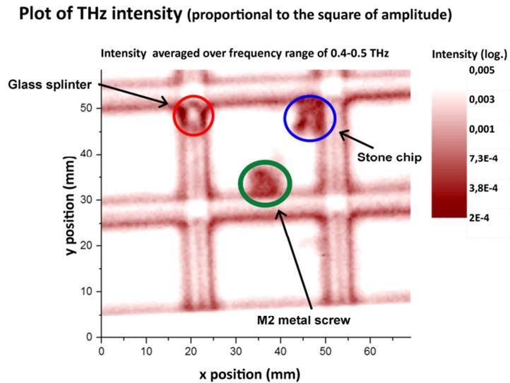
**Fig. 4:** THz intensity image of a chocolate bar with different contaminating particles (compare Fig. 3).
