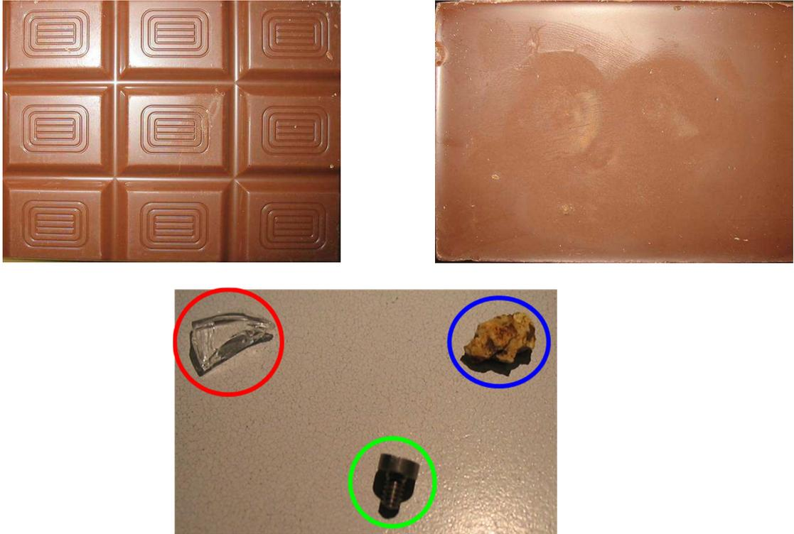
**Fig. 3:** Front and back side of chocolate bar after preparation with a glass splinter, a stone, and a metal screw.
