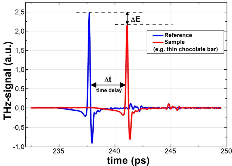
**Fig. 2:** THz pulses measured in air reference (blue) and in a thin chocolate sample (red). The temporal position is shifted and the amplitude is decreased after the chocolate.
