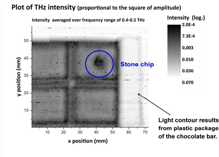
**Fig. 5:** THz intensity image of a chocolate bar wrapped in plastic foil. The dark area in the upper corner is resulting from the stone.
