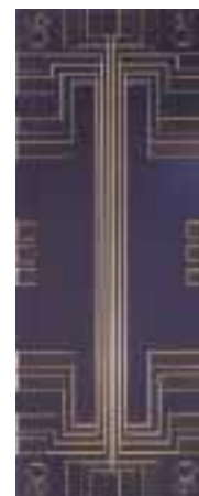
Tera8 - 6 dipole structures on each chip
