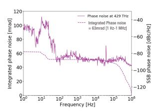
Analysis of the out of loop beat signal between two  $\text{ULN}^{\text{plus}}$  combs at the Strontium clock transition frequency:
