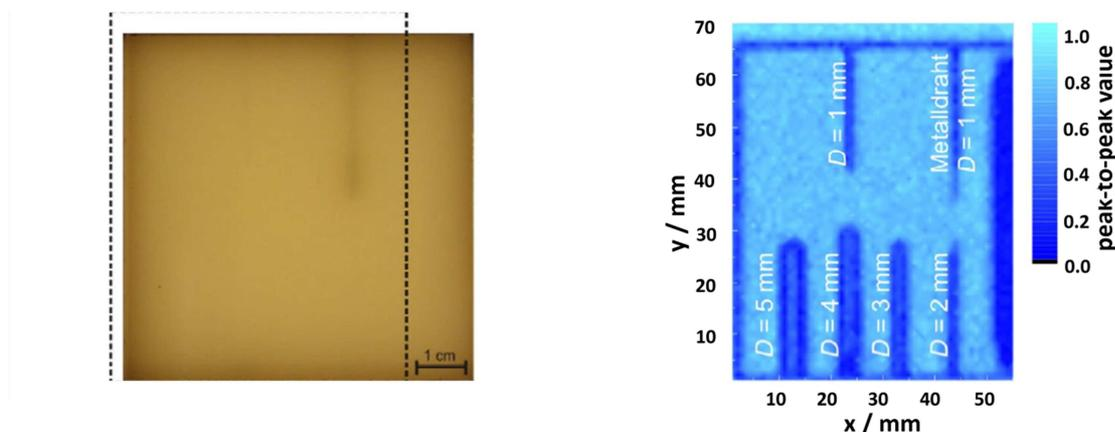
**Fig. 2:** Left part: Backlight picture of two welded plastic slabs (PE) with simulated delamination. Right part: THz transmission image where darker areas indicate delamination defects, e.g. metal impurities, here represented by a wire („Metalldraht“).
