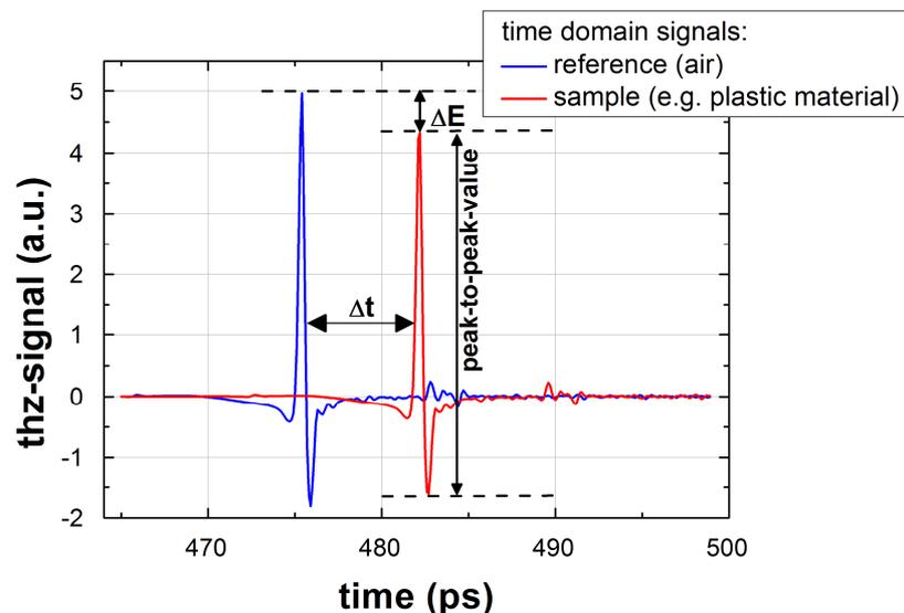
**Fig.1:** Time traces of THz pulses measured in air (reference, blue line) and after transmission through a 2 mm thick polypropylene (PP) slab (sample, red line). The amplitude of the sample pulse is decreased by  $\Delta E$  due to absorption in the material and the temporal position of the THz pulse is shifted due to dispersion ( $\Delta t$ ).
