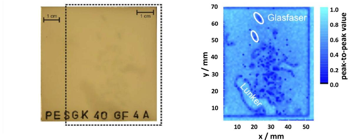
**Fig. 3:** Two plastic slabs (PE) glued together. Left part: The black frame on the photo defines the imaged area. Right part: THz transmission image with darker areas showing impurities such as a blowhole (“Lunker”) or pieces of glass fiber (“Glasfaser”).
