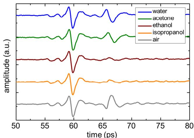
**Figure 4:** THz traces of various fluids, showing the first and the second pulse reflected off the air/container and container/fluid interface, respectively
